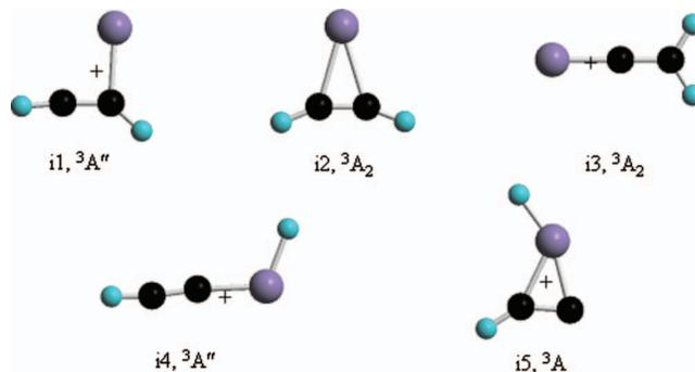
FIG. 5. Structures of various triplet  $\text{SiC}_2\text{H}_2$  reaction intermediates potentially formed in the reaction of ground state silicon atoms with acetylene as extracted from Ref. 15. The location of the rotational axis located perpendicular to the paper plane, which would lead to  $B$ -like rotations in the linear  $\text{SiCCH}(X^2\Pi)$  radical, is defined as + and was derived from the geometries of the intermediates as calculated by Talbi.
