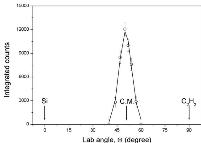
FIG. 2. Laboratory angular distribution of ions extracted from ions at mass-to-charge ratio  $m/z$  of 53 ( $\text{SiC}_2\text{H}^+$ ) in the crossed beam reaction of ground state silicon atoms ( $\text{Si}(^3\text{P})$ ) with acetylene ( $\text{C}_2\text{H}_2$ ) at a collision energy of  $101.6 \text{ kJ mol}^{-1}$ . The circles are the experimental data and the solid lines the best fits utilizing the CM functions depicted in Fig. 3.
