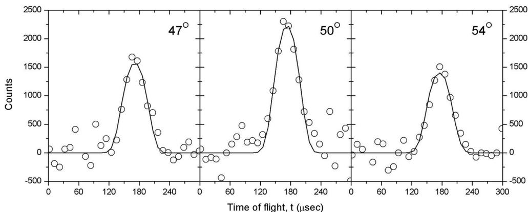
FIG. 1. Selected TOF spectra recorded at a mass-to-charge ratio  $m/z$  of 53 ( $\text{SiC}_2\text{H}^+$ ) in the crossed beam reaction of ground state silicon atoms ( $\text{Si}(^3\text{P})$ ) with acetylene ( $\text{C}_2\text{H}_2$ ) at a collision energy of  $101.6 \text{ kJ mol}^{-1}$ . The circles are the experimental data and the solid lines are the best fits utilizing the CM functions depicted in Fig. 3. Up to  $8 \times 10^6$  TOF were accumulated per angle.
