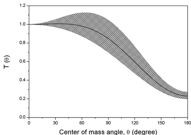
FIG. 3. CM translational energy (top) and angular (bottom) distributions of the linear  $\text{SiCCH}(X^2\Pi)$  radical formed in the reaction of ground state silicon atoms with acetylene. The solid lines represent the best fits and the hatched areas represent the allowable fits within the experimental error limits.
