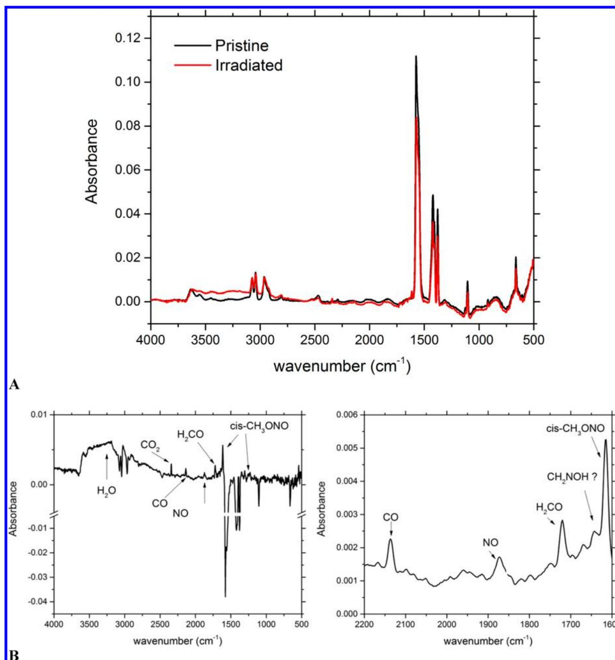
**Figure 2.** (A) Infrared spectra of the nitromethane ices at 5.5 K before (black) and after (red), irradiation at 15 nA. (B) Difference spectra of pristine and irradiated nitromethane ice at 5.5 K to highlight the subtle changes; shown on the right is an expanded view for clarity.
