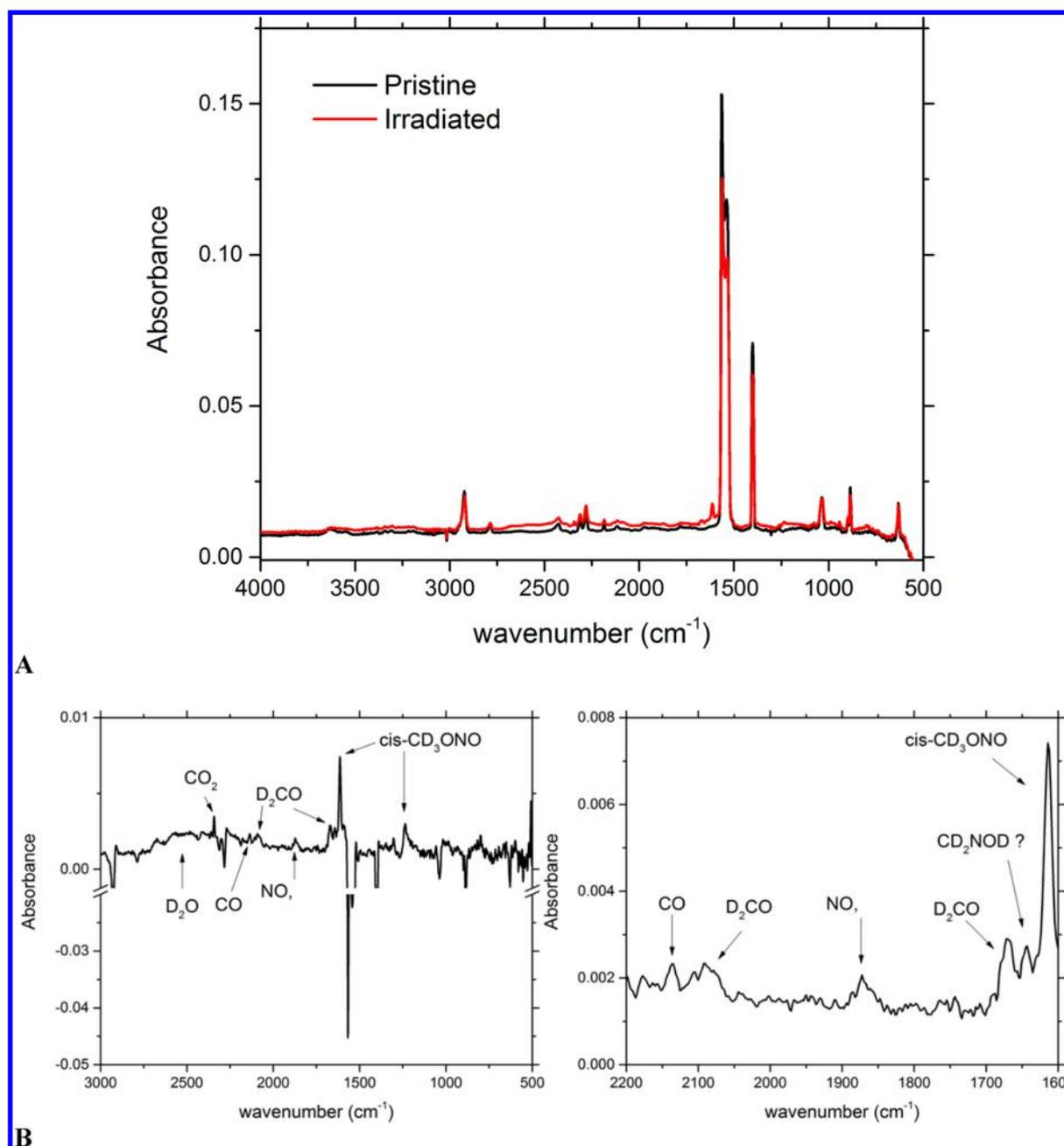
**Figure 3.** (A) Infrared spectra of the D3-nitromethane ( $\text{CD}_3\text{NO}_2$ ) ices at 5.5 K before (black) and after (red) irradiation at 15 nA. (B) Difference spectra of pristine and irradiated D3-nitromethane ice at 5.5 K to highlight the subtle changes; shown on the right is an expanded view for clarity.
