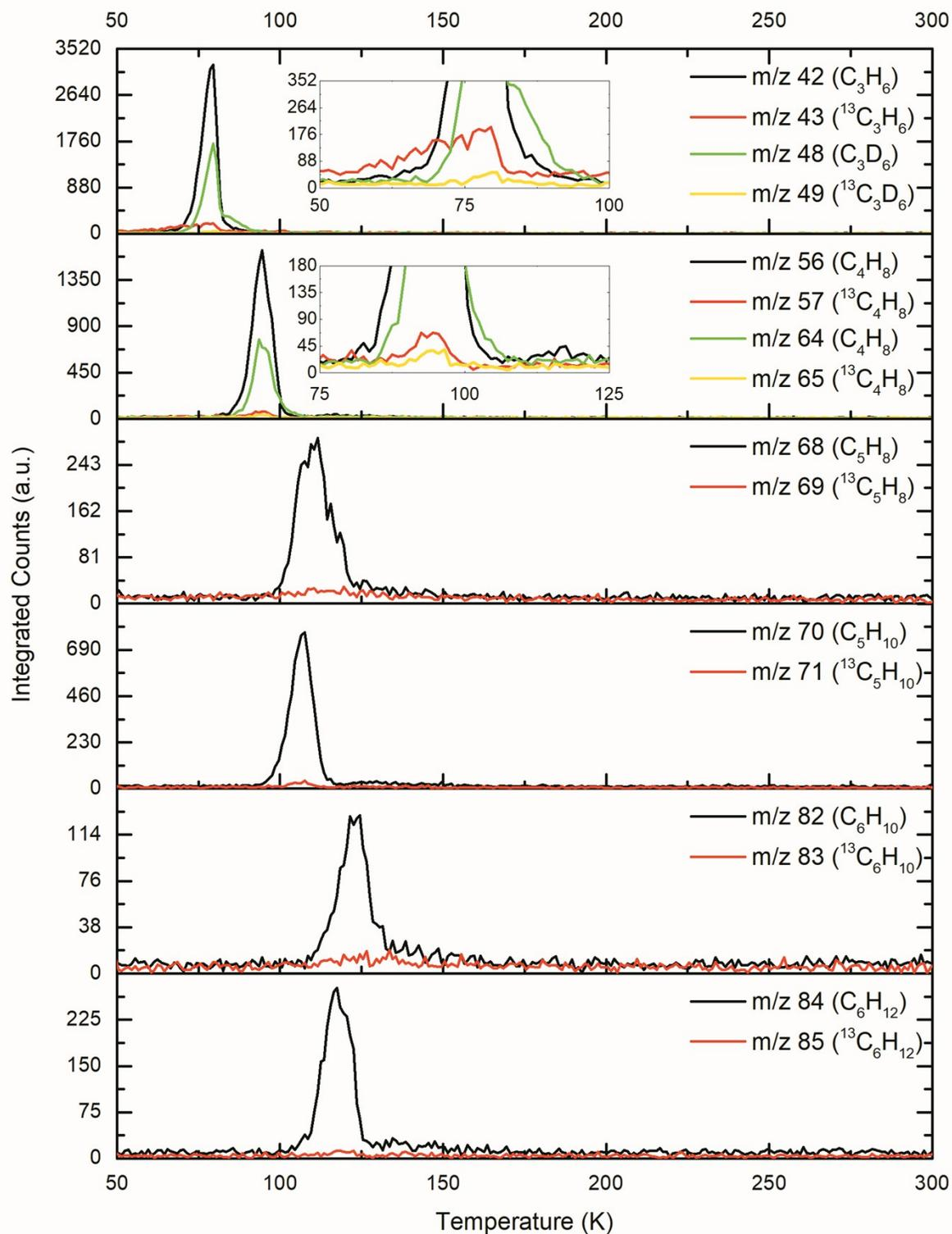
Figure S9. Overlay of TPD profiles after electron irradiation of products from methane ( $\text{CH}_4$ ; black) and D4-methane ( $\text{CD}_4$ ; green) ices with prospective  $^{13}\text{C}$  isotopologues (red and yellow, respectively).
