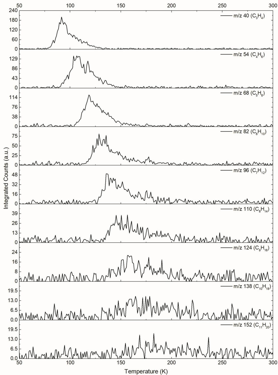
Figure S5. TPD profiles recorded after Lyman  $\alpha$  photolysis via PI-ReTOF-MS for masses with the generic formula of  $C_nH_{2n-2}$  (alkynes, dienes, and/or cycloalkenes).
