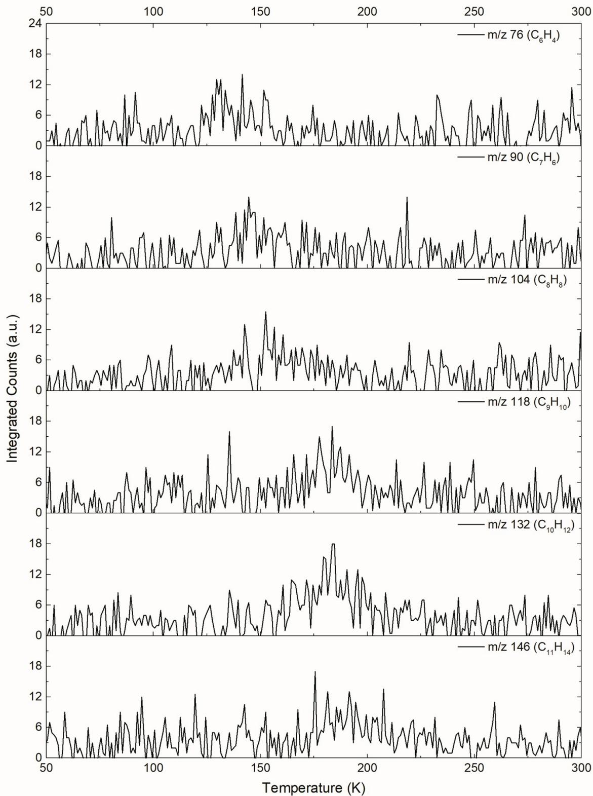
Figure S8. TPD profiles recorded after Lyman  $\alpha$  photolysis via PI-ReTOF-MS for masses with the generic formula of  $C_nH_{2n-8}$  (yne-triene, diyne-ene, pentaenes, tri-cyclobialkenes).
