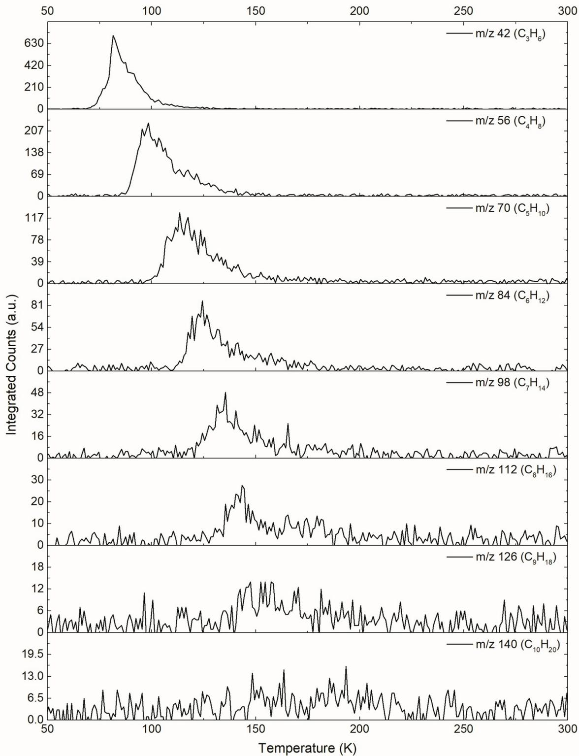
Figure S4. TPD profiles recorded after Lyman  $\alpha$  photolysis via PI-ReTOF-MS for masses with the generic formula of  $C_nH_{2n}$  (alkenes and/or cycloalkanes).
