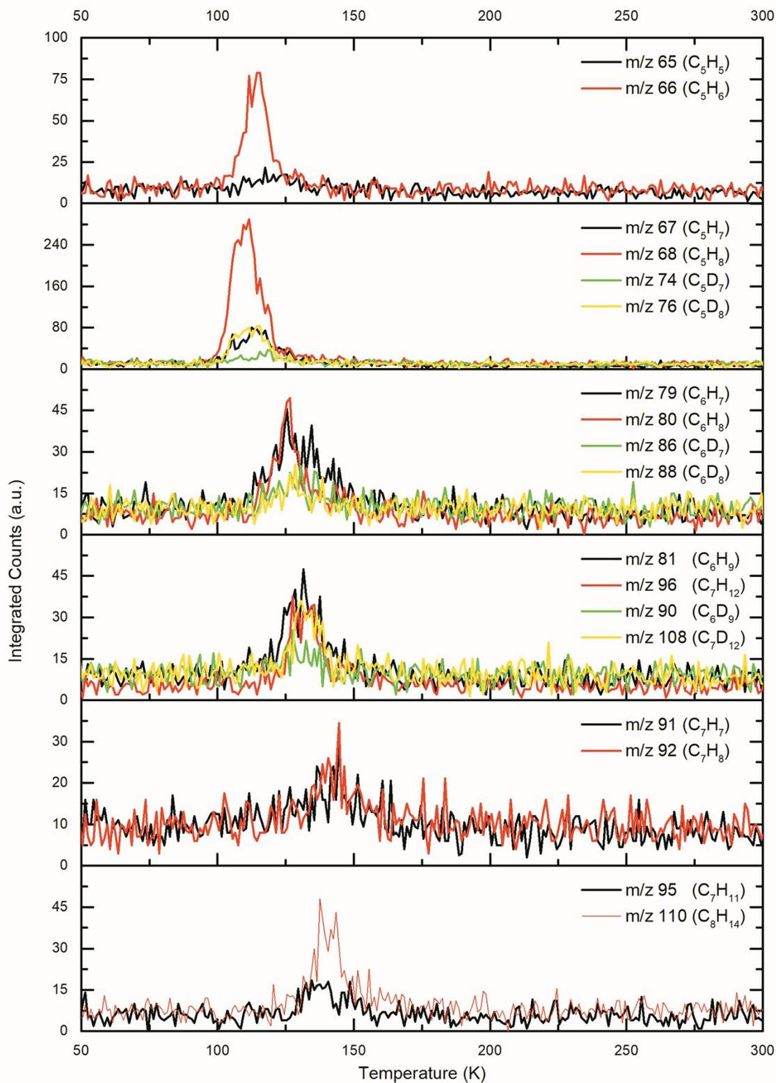
Figure S10. TPD profiles after electron irradiation of ions corresponding to fragments from methane ( $\text{CH}_4$ ; black) and D4-methane ( $\text{CD}_4$ ; green) ice from a larger parent molecule (red and yellow, respectively).
