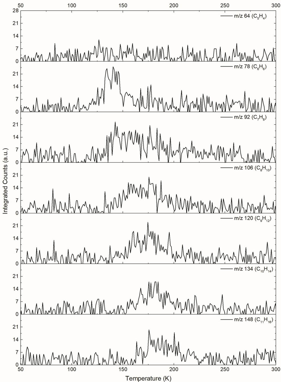
Figure S7. TPD profiles recorded after Lyman  $\alpha$  photolysis via PI-ReTOF-MS for masses with the generic formula of  $C_nH_{2n-6}$  (yne-diene, diyne, tetraene, cyclotrialkenes, tri-cycloalkenes).
