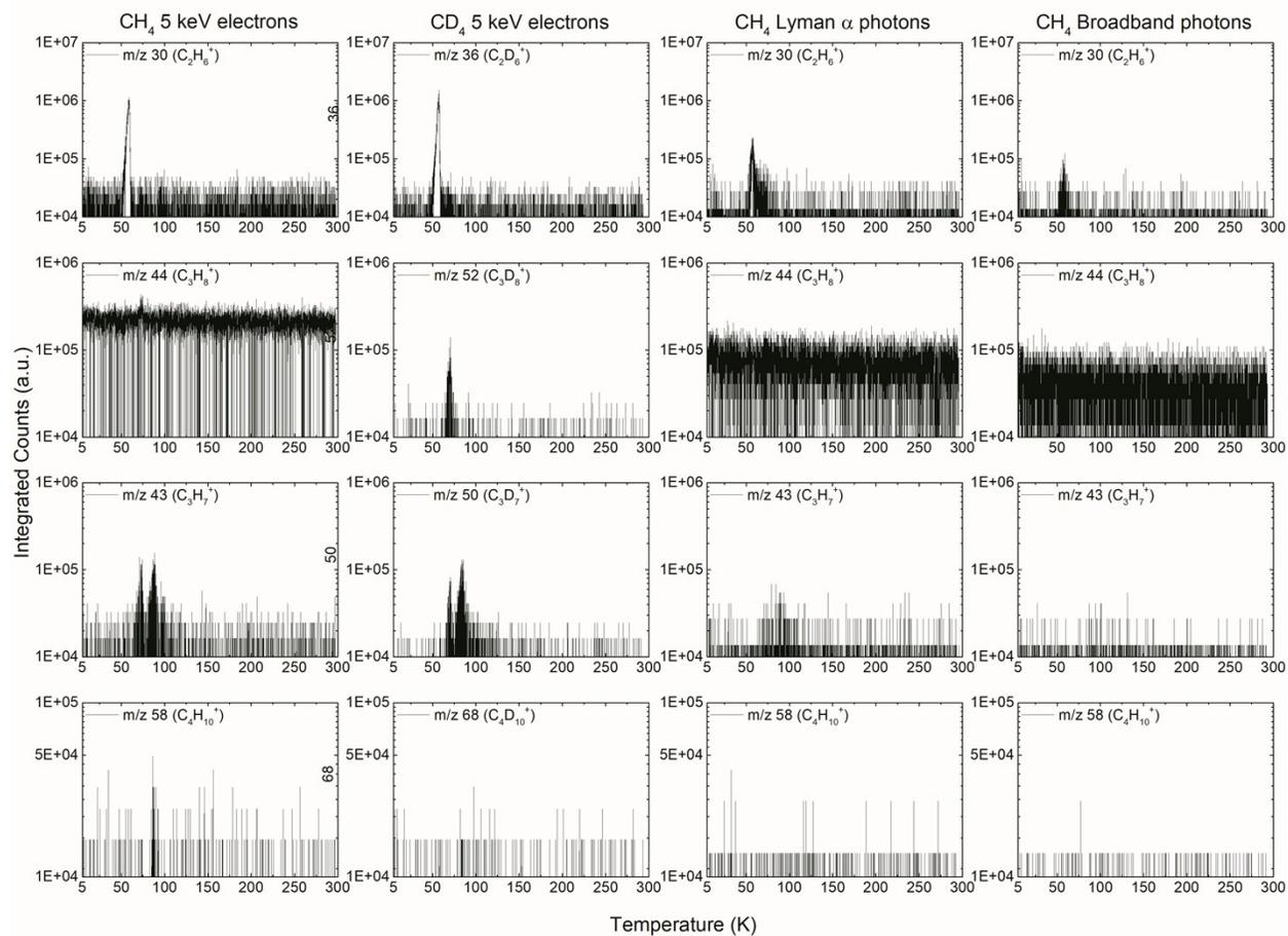
Figure S2. Sublimation profiles recorded during temperature programmed desorption via the RGA for ethane (C<sub>2</sub>H<sub>6</sub>/C<sub>2</sub>D<sub>6</sub>), propane (C<sub>3</sub>H<sub>8</sub>/C<sub>3</sub>D<sub>8</sub>), the C<sub>3</sub>H<sub>7</sub><sup>+</sup> fragment, and butane (C<sub>4</sub>H<sub>10</sub>/C<sub>4</sub>D<sub>10</sub>) from the electron irradiation (first and second columns), Lyman α photolysis (third column), and broadband photolysis (fourth column).
