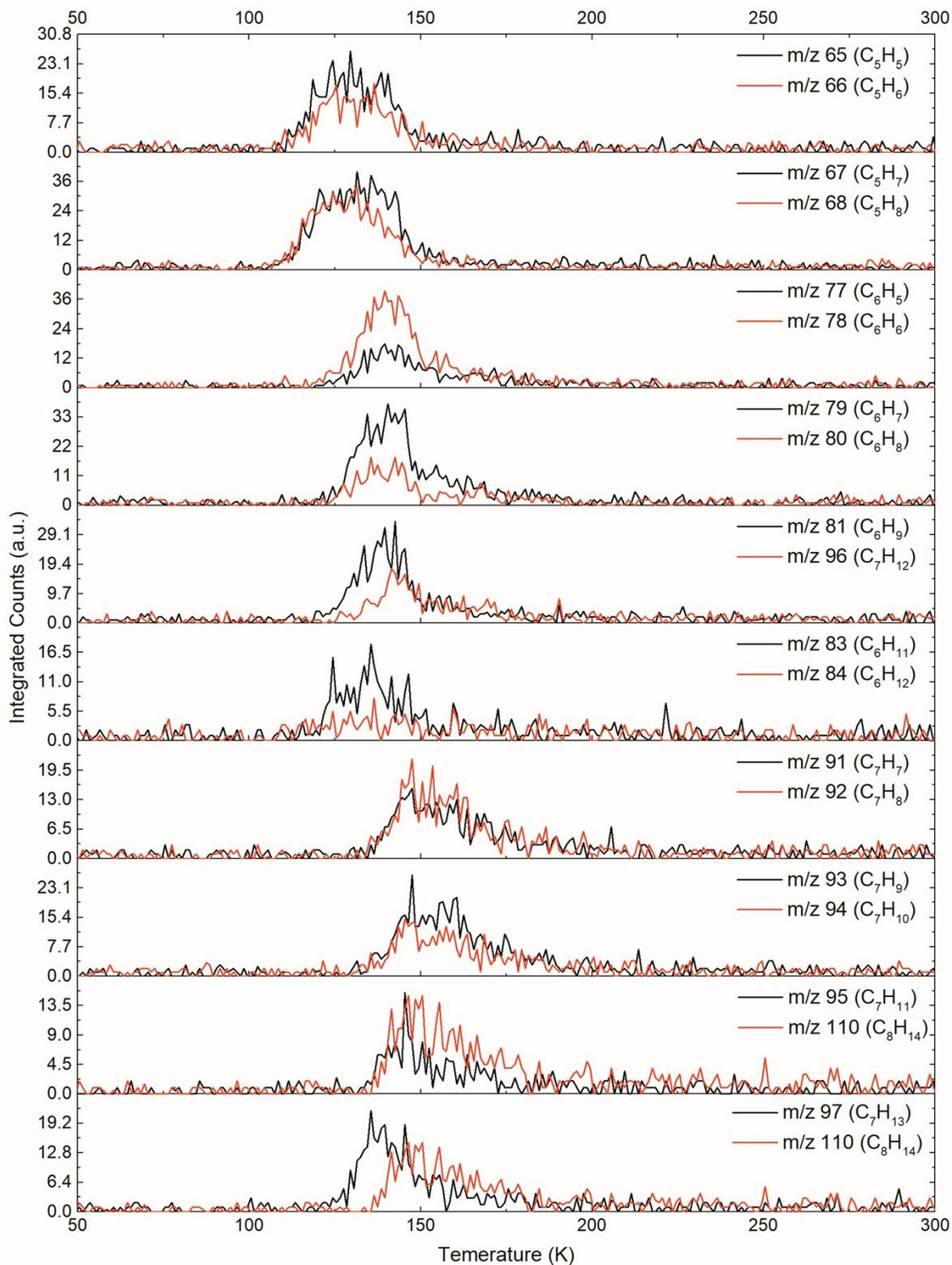
Figure S11. TPD profiles after broadband photolysis of ions corresponding to fragments from methane ( $\text{CH}_4$ ; black) ice from a larger parent molecule (red).
