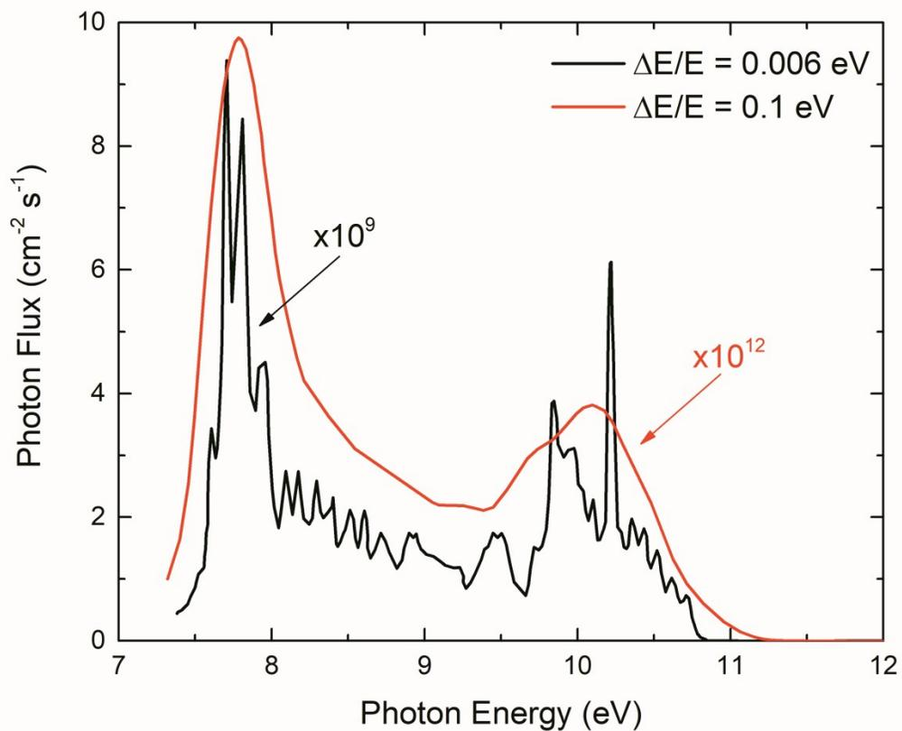
Figure S1. The photon flux profile of the continuous wave VUV photolysis source coupled to a monochromator and light collimation chamber at high (black) and low (red) resolution from 7.3-11.0 eV using a NIST calibrated photodiode.
