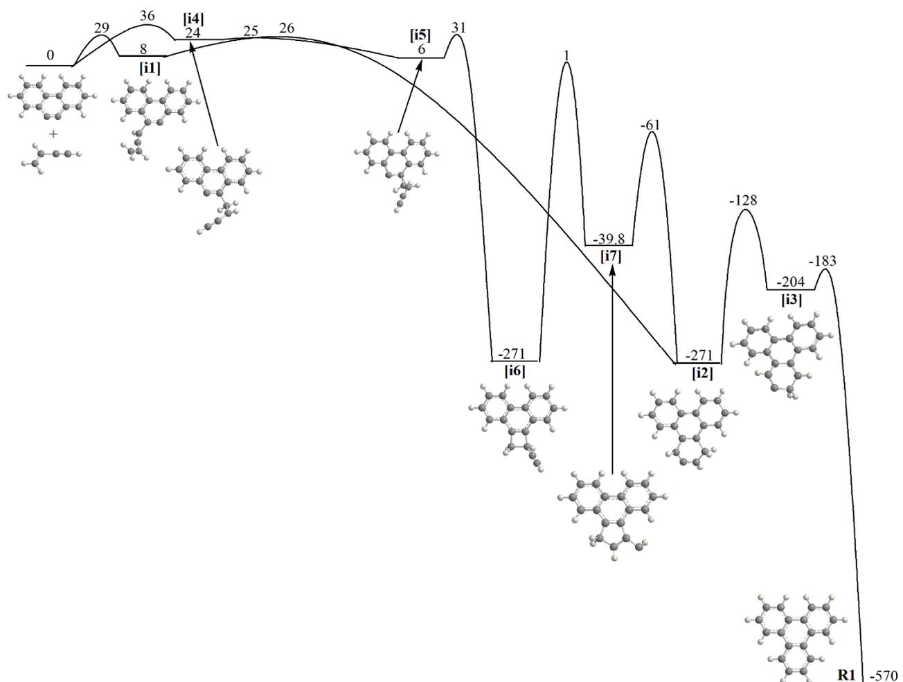
**Figure S4.** PES for the phenanthryne ( $C_{14}H_8$ ) reaction with vinylacetylene ( $C_4H_4$ ) calculated at the B3LYP/6-311G(d,p) level of theory. The relative energies are given in  $\text{kJ mol}^{-1}$ .
