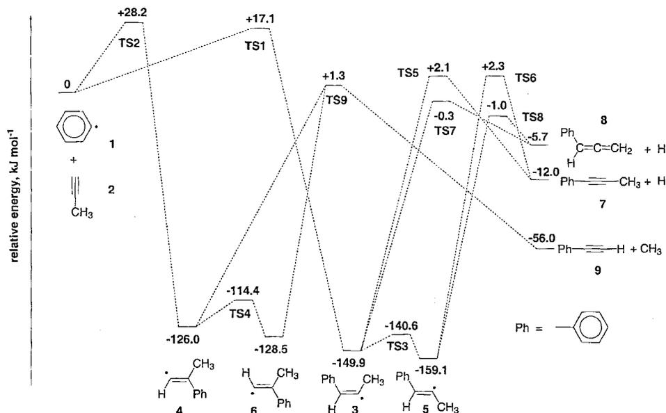
FIG. 6. Schematic representation of the  $C_9H_9$  potential energy surface at the B3LYP/6-311+G\*\* level of theory. Computational details are given in the text.
