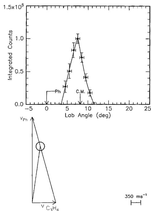
FIG. 2. Laboratory angular distribution together with the most probable Newton diagram for the  $C_6H_5(X^2A') + CH_3CCH(X^1A_1)$  reaction at a collision energy of  $140 \text{ kJ mol}^{-1}$ . The circle centrosymmetric around the center of mass stands for the maximum center-of-mass recoil velocity of the phenylmethylacetylene product.
