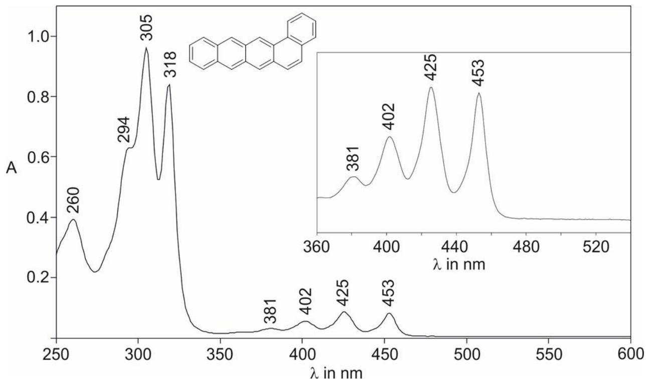
**Figure S11:** Absorption spectrum of benzo[*a*]tetracene (compound **P2**) in  $\text{CHCl}_3$  ( $c=1.65 \times 10^{-5}$  mol/l).
