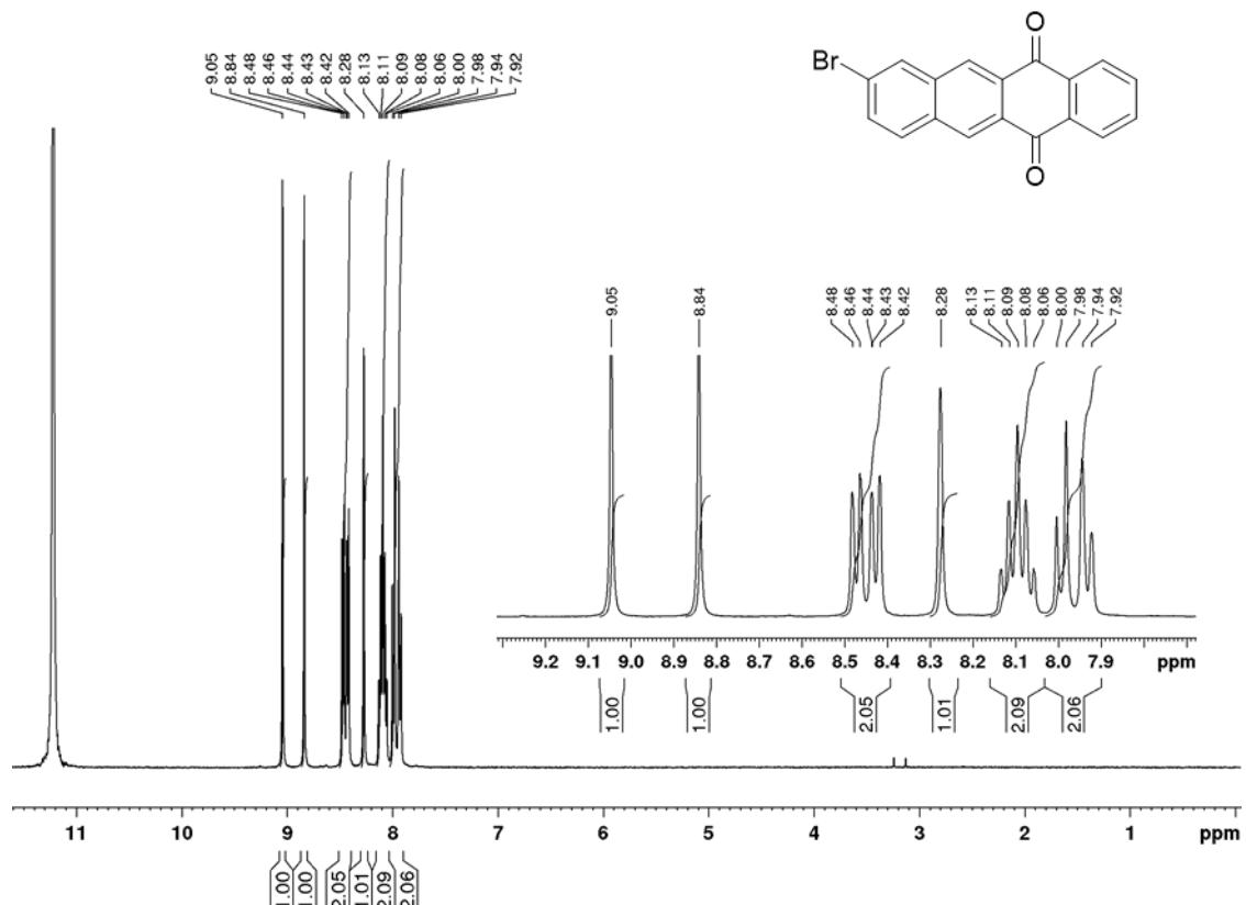
**Figure S2:** <sup>1</sup>H NMR spectrum of 8-bromotetracene-5,12-dione (compound 3) in D<sub>2</sub>SO<sub>4</sub>.
