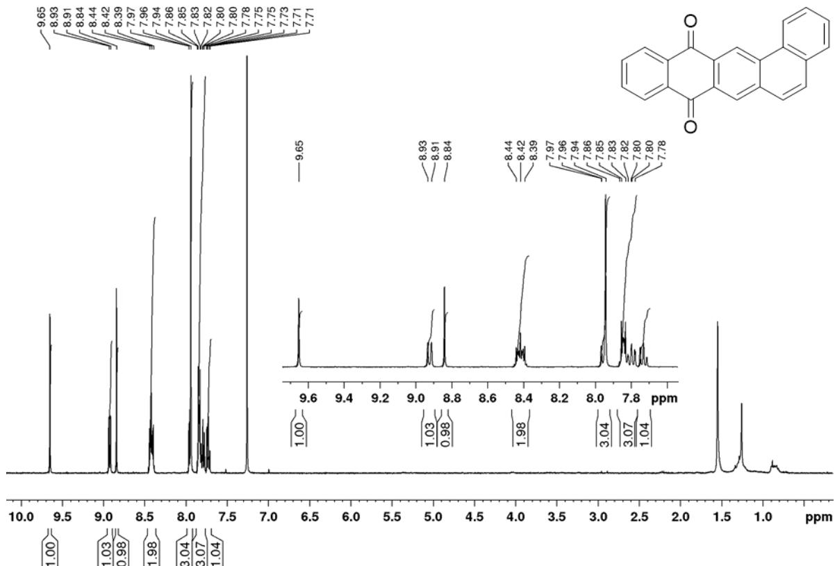
**Figure S6:**  $^1\text{H}$  NMR spectrum of benzo[*a*]tetracene-8,13-dione (compound 7) in  $\text{CDCl}_3$ .
