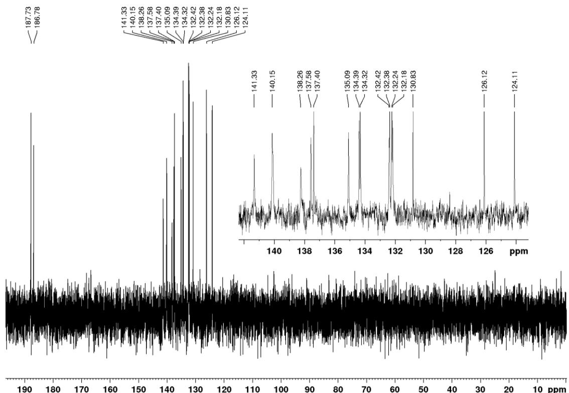
**Figure S3:** <sup>13</sup>C NMR spectrum of 8-bromotetracene-5,12-dione (compound 3) in D<sub>2</sub>SO<sub>4</sub>.
