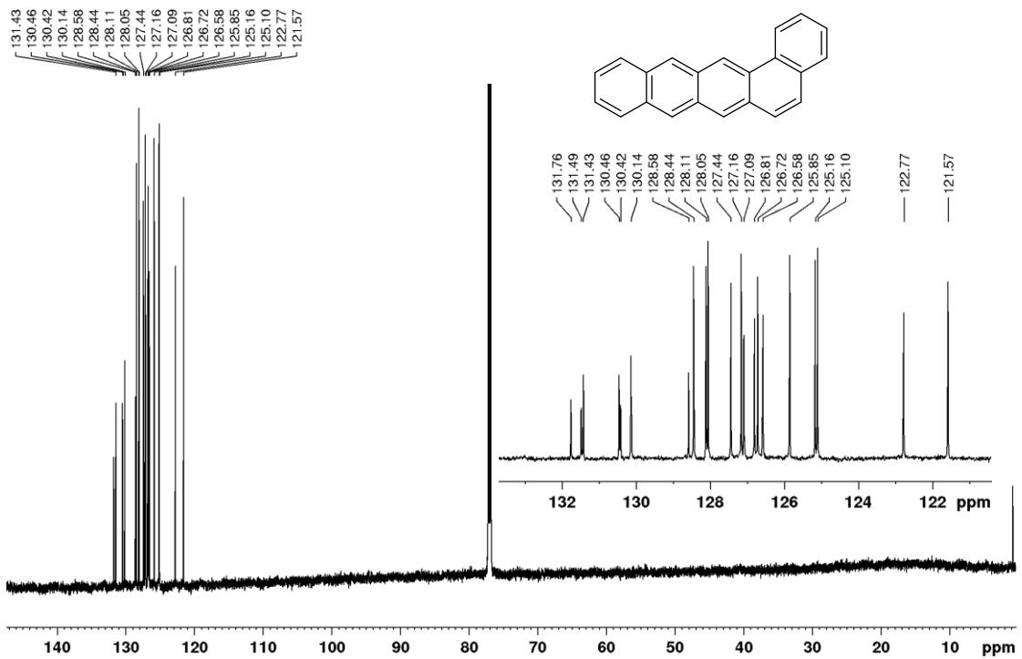
**Figure S9:**  $^{13}\text{C}$  NMR spectrum of benzo[*a*]tetracene (compound **P2**) in  $\text{CDCl}_3/\text{CS}_2$ .
