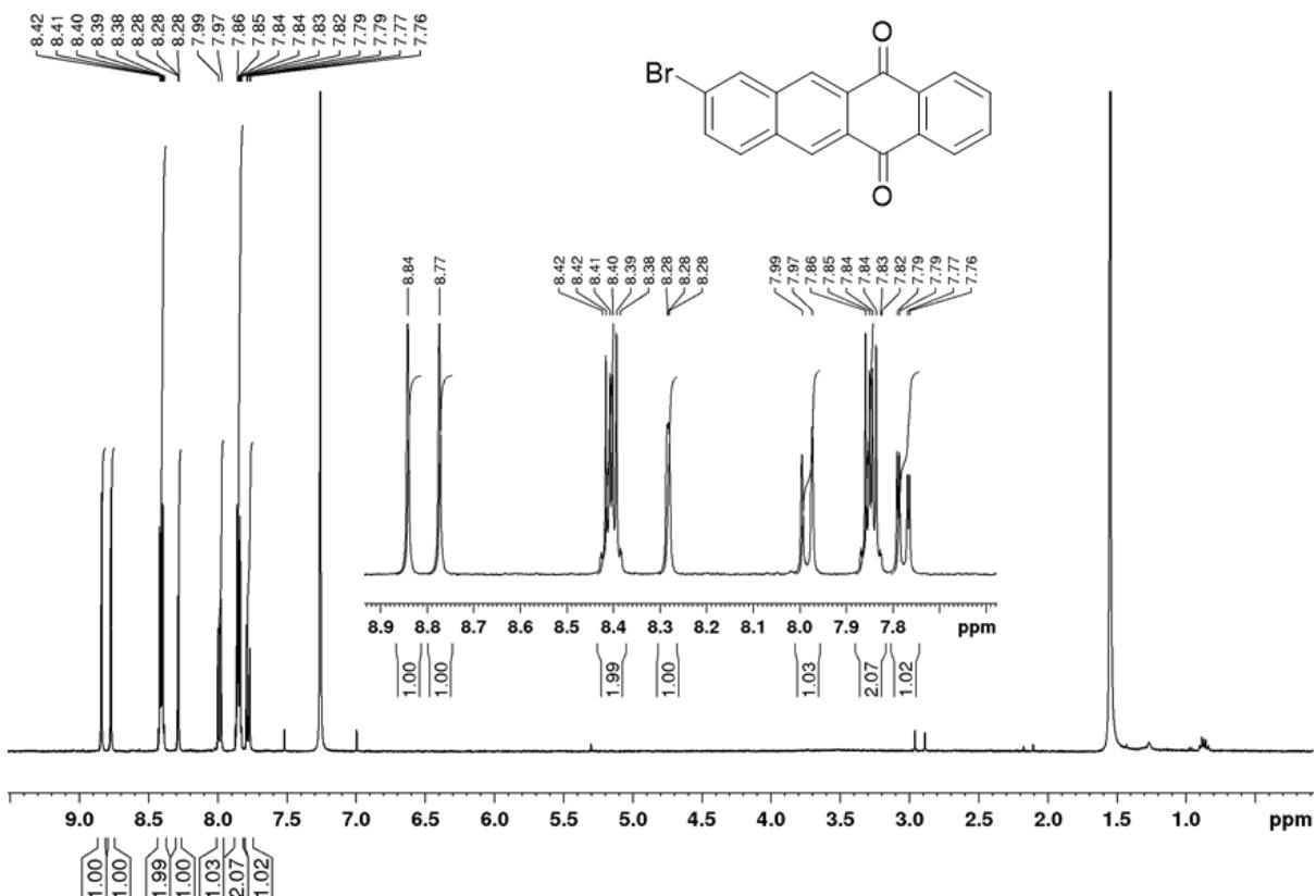
**Figure S4:**  $^1\text{H}$  NMR spectrum of 8-bromotetracene-5,12-dione (compound 3) in  $\text{CDCl}_3$ .
