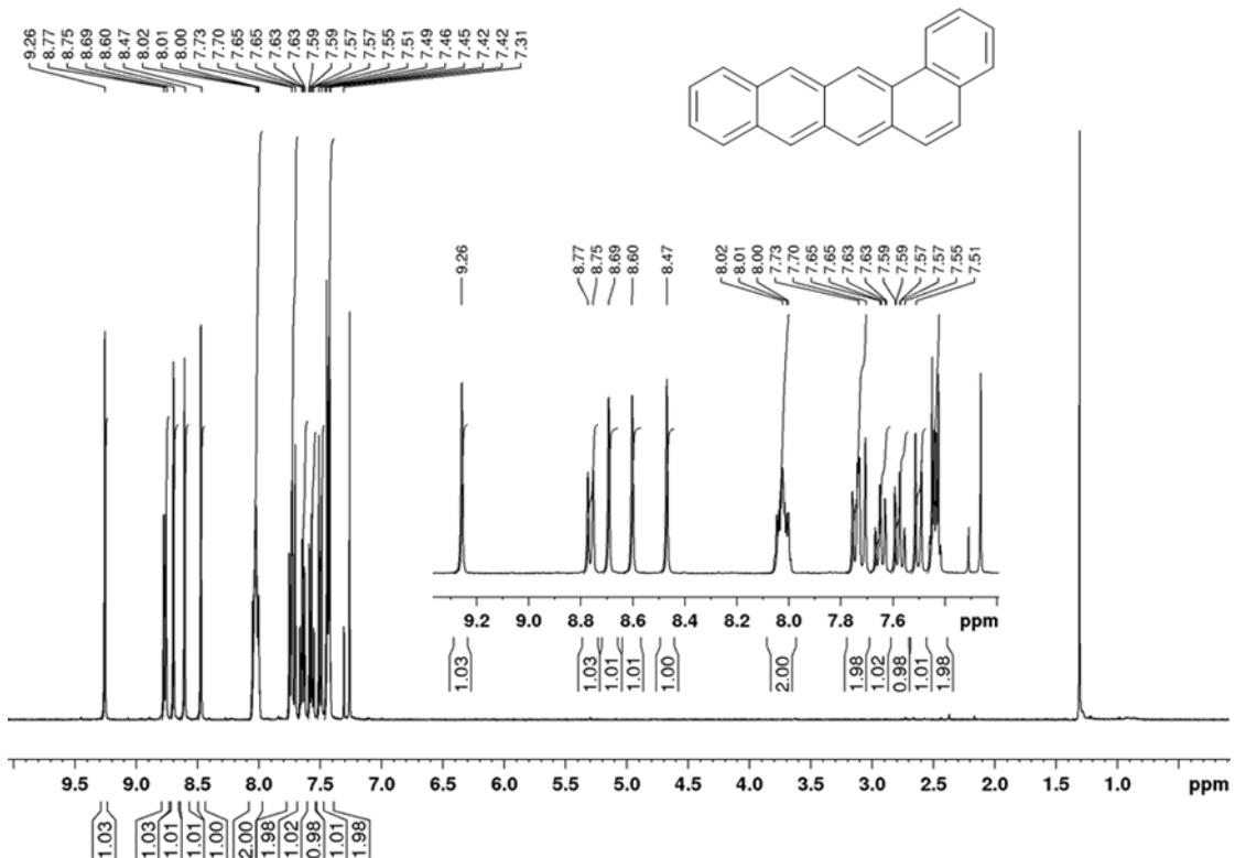
**Figure S8:**  $^1\text{H}$  NMR spectrum of benzo[*a*]tetracene (compound **P2**) in  $\text{CDCl}_3/\text{CS}_2$ ; the peak at 7.31 ppm is due to an impurity in  $\text{CS}_2$ .
