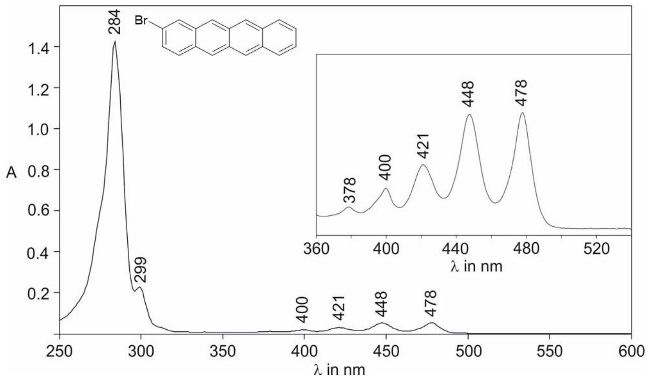
**Figure S10:** Absorption spectrum of 2-bromotetracene (compound **4**) in  $\text{CHCl}_3$ .
