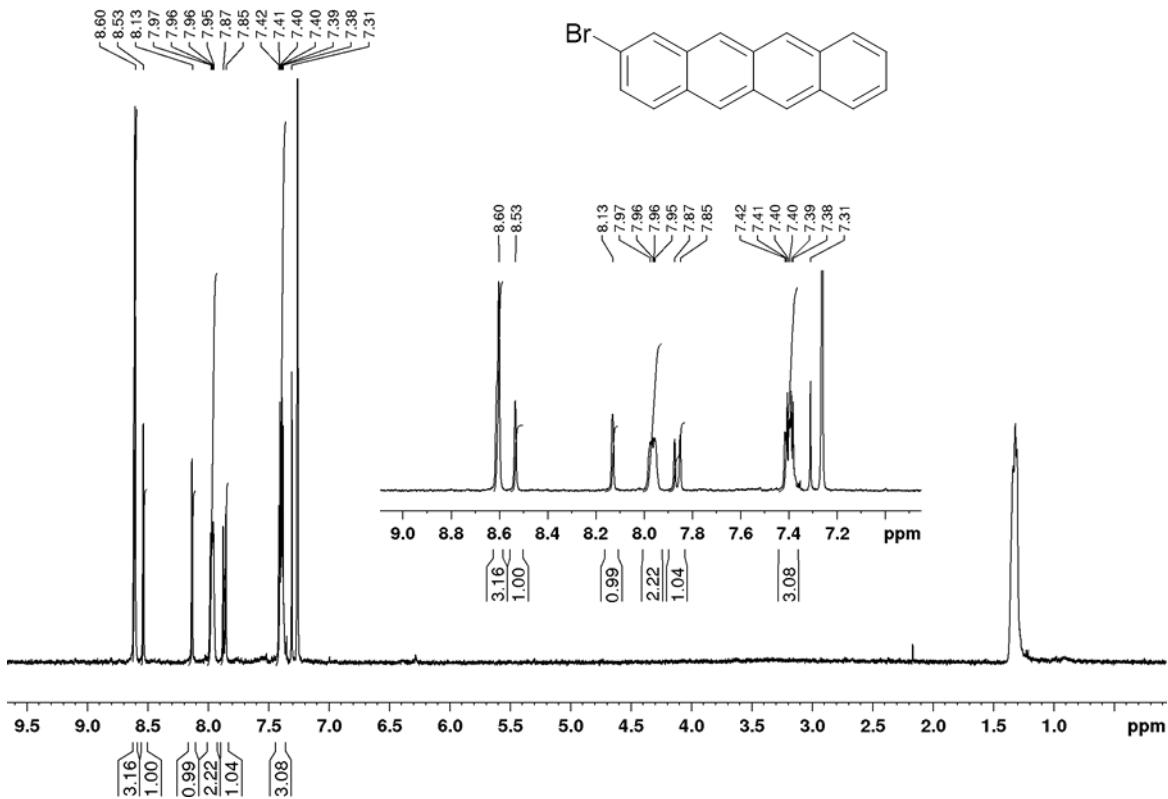
**Figure S5:**  $^1\text{H}$  NMR spectrum of 2-bromotetracene (compound 4) in  $\text{CDCl}_3/\text{CS}_2$ ; the peak at 7.31 ppm is due to an impurity in the  $\text{CS}_2$ .
