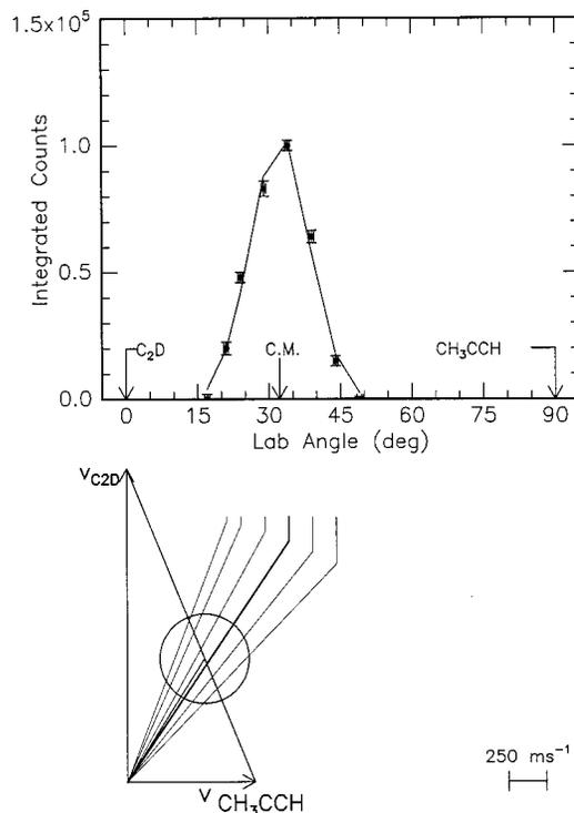
FIG. 2. Laboratory angular distribution together with the most probable Newton diagram for the  $\text{C}_2\text{D}(X^2\Sigma^+) + \text{CH}_3\text{CCH}(X^1A_1)$  reaction at a collision energy of  $39.8 \text{ kJ mol}^{-1}$ . The circle centrosymmetric around the center of mass stands for the maximum center-of-mass recoil velocity of the methylidyne,  $\text{CH}_3\text{CCCD}$ , product.
