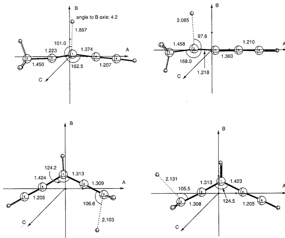
FIG. 8. Structure of four exit transition states from **5** to  $\text{CH}_3\text{CCCCH}$  (top left), **8** to  $\text{CH}_3\text{CCCCH}$  (top right), **3** to  $\text{H}_2\text{CCCH}(\text{C}_2\text{H})$  (bottom left), and **5** to  $\text{H}_2\text{CCCH}(\text{C}_2\text{H})$  (bottom right). Bond distances are given in Å and bond angles in deg.
