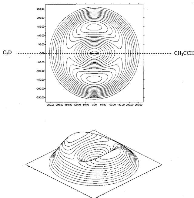
FIG. 5. Center-of-mass velocity contour flux map distribution for the  $C_2D(X^2\Sigma^+) + CH_3CCH(X^1A_1)$  reaction at a collision energy of  $39.8 \text{ kJ mol}^{-1}$ ; top: two-dimensional view, bottom: three-dimensional view. The contour lines connect data points with an identical flux. Units of the  $x$  and  $y$  axes are given in  $\text{ms}^{-1}$ .
