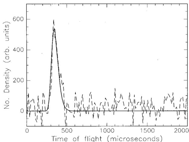
FIG. 3. Time-of-flight data at  $32.5^\circ$  for the  $C_2D(X^2\Sigma^+) + CH_3CCH(X^1A_1)$  reaction at a collision energy of  $39.8 \text{ kJ mol}^{-1}$ . The dashed line indicates the experimental data, the solid line the calculated fit.
