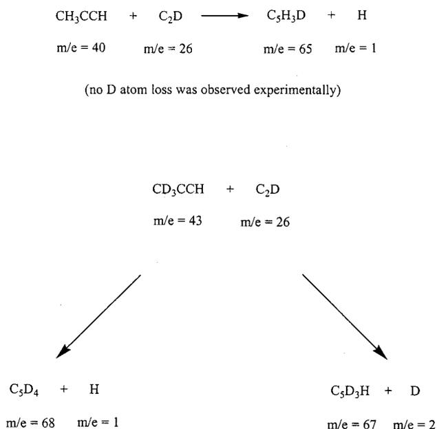
FIG. 1. Schematic representation of the mass to charge ratios of the H and D atom exchange pathway in the reaction of the  $\text{C}_2\text{D}(X^2\Sigma^+)$  with  $\text{CH}_3\text{CCH}(X^1A_1)$  at a collision energy of  $39.8 \text{ kJ mol}^{-1}$ .
