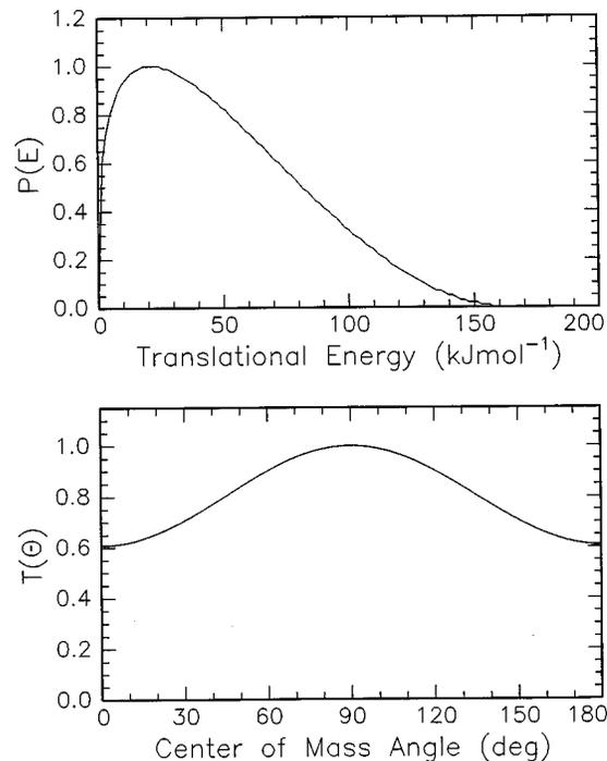
FIG. 4. Center-of-mass angular flux distribution (lower) and translational energy flux distribution (upper) for the  $C_2D(X^2\Sigma^+) + CH_3CCH(X^1A_1)$  reaction at a collision energy of  $39.8 \text{ kJ mol}^{-1}$ .
