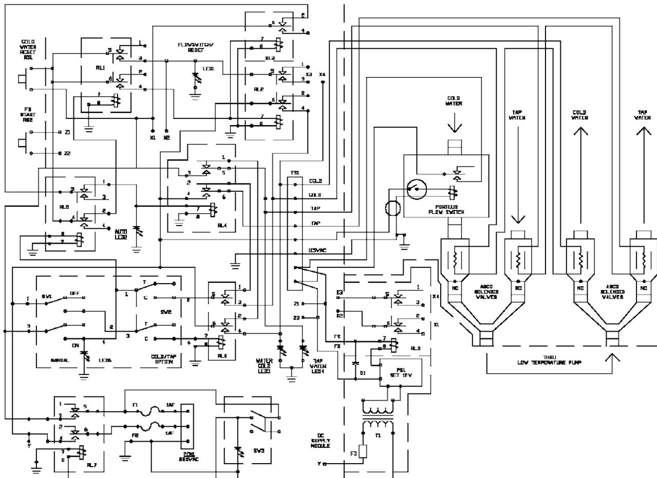
FIG. 4. Circuit diagram of the water flow interlock module.
