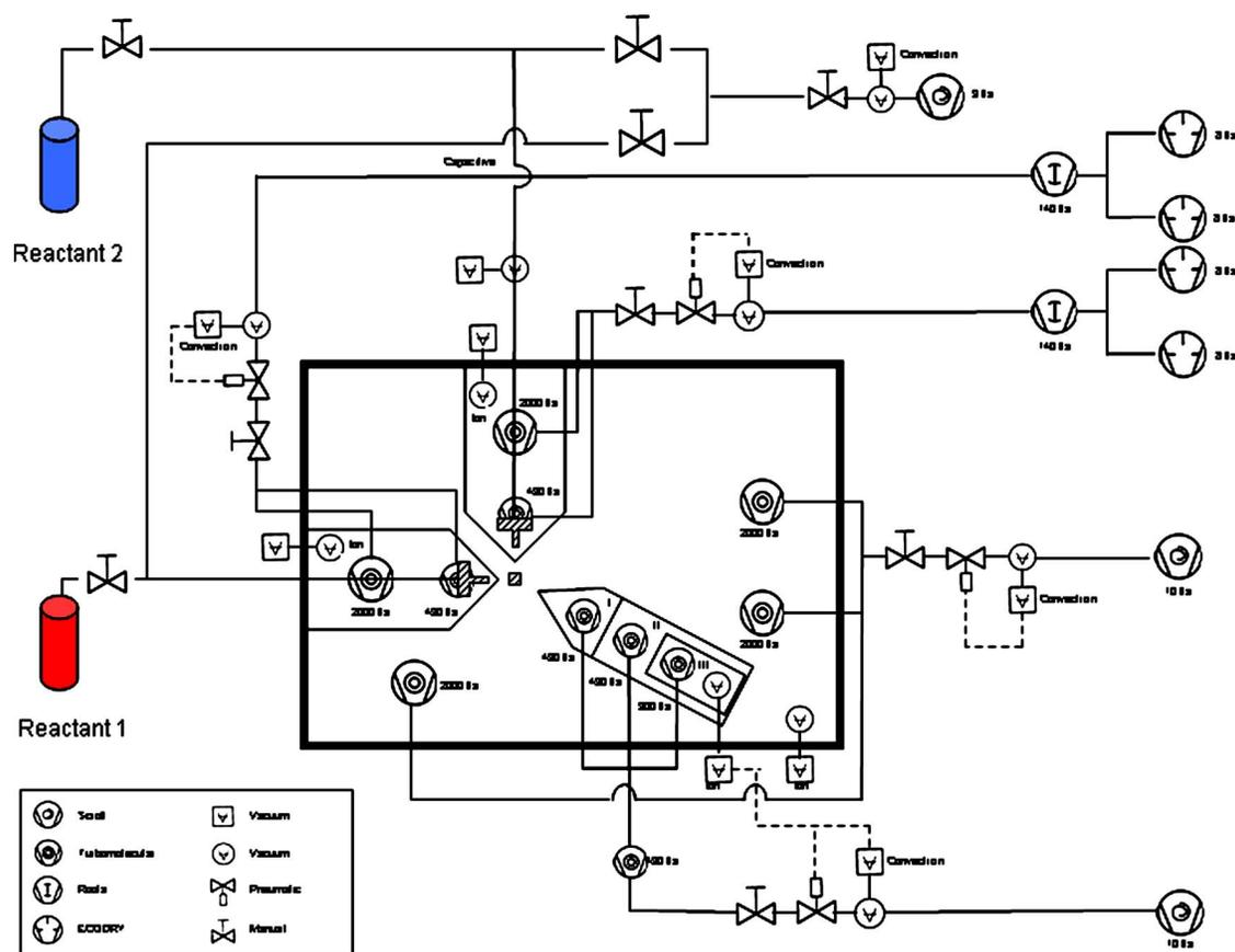
FIG. 1. Pumping scheme of the crossed beams machine. Chopper wheels are omitted for clarity.
