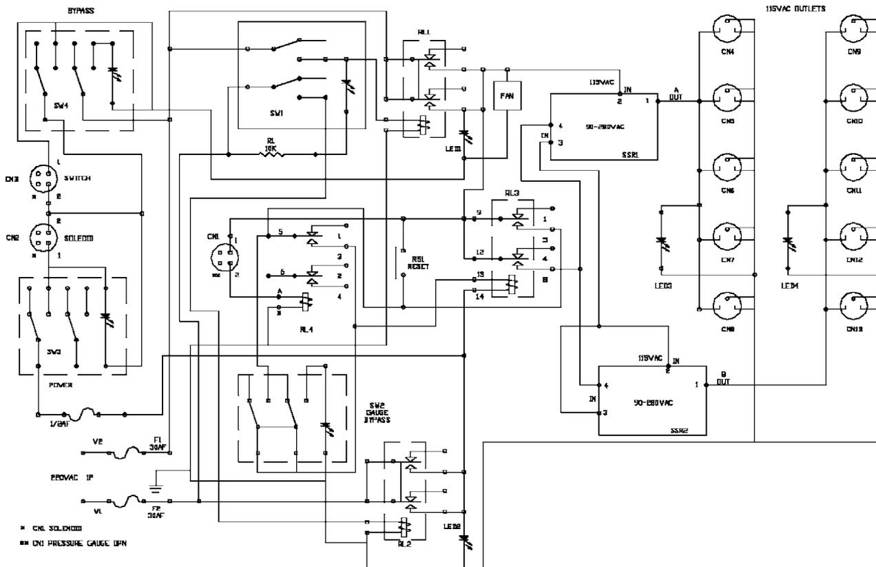
FIG. 3. Circuit diagram of the detector vacuum interlock module.
