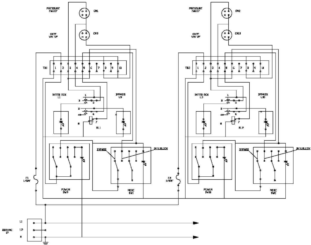
FIG. 2. Circuit diagram of one unit of the main chamber vacuum interlock module.
